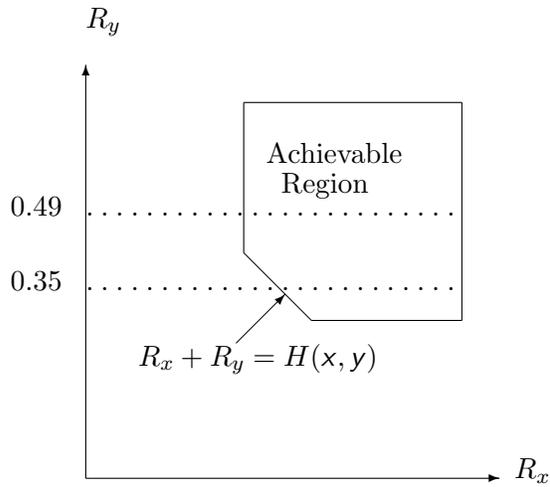
Figure 5: Rate region for the example 2 source, we focus on the error exponent on source  $x$  for fixed encoder  $y$  rates:  $R_y = 0.35$  and  $R_y = 0.49$
