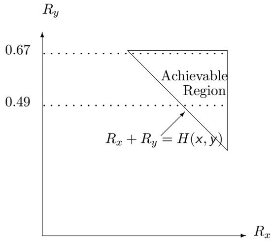
Figure 3: Rate region for the example 1 source, we focus on the error exponent on source  $x$  for fixed encoder  $y$  rates:  $R_y = 0.49$  and  $R_y = 0.67$
