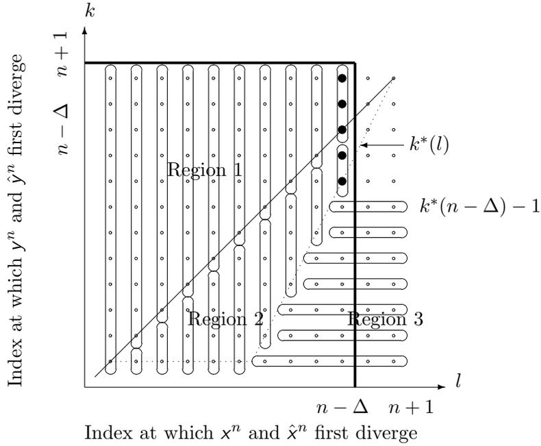
Figure 10: Two dimensional plot of the error probabilities  $p_n(l, k)$ , corresponding to error events  $(l, k)$ , contributing to  $\Pr[\hat{x}^{n-\Delta} \neq x^{n-\Delta}]$  in the situation where  $\inf_{\gamma \in [0,1]} E_y(R_x, R_y, \gamma) < \inf_{\gamma \in [0,1]} E_x(R_x, R_y, \gamma)$ .
