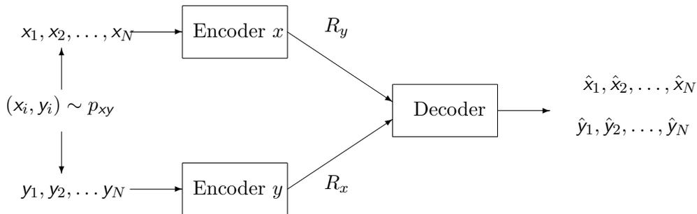
Figure 1: Slepian-Wolf distributed encoding and joint decoding of a pair of correlated sources.
